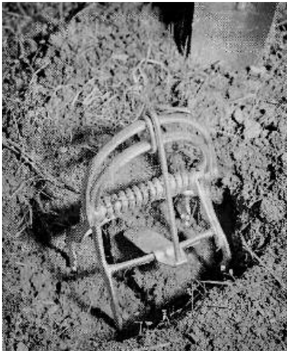
Fig. 3. Jaw type mole trap set in excavated hole to straddle mole run.
