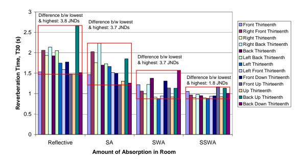
Figure 4 – Reverberation time results for each of the **thirteenth** sources for each level of absorption in the model.
