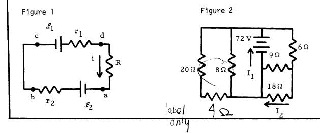
B(1, 2). For the circuit shown in Figure 2 find the equivalent resistance of the resistance network, and find currents  $I_1$  and  $I_2$ .
