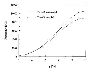
Fig. 4(a). Frequency of flame oscillation  $T_{y} = 600 \text{ K}$ .
