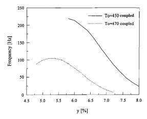
Fig. 5. Frequency of flame oscillation Le = 1.5
