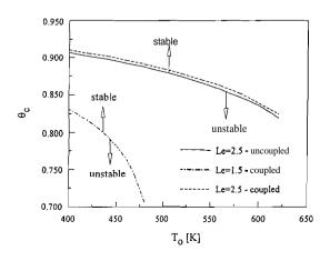
Fig. 2. Critical temperature (6% methane)
