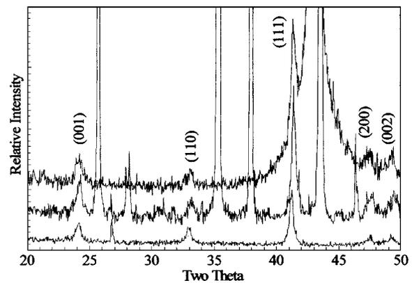
FIG. 3. X-ray diffraction patterns of FePt films deposited on (100) MgO (top), polycrystalline Al<sub>2</sub>O<sub>3</sub> (middle), and (001) Si (bottom). All films have been heat treated at 600 °C for 10 min. The presence of the (001) and (110) peaks, as well as the splitting of the {002}, indicates that the  $L1_0$  structure has formed.
