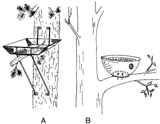
**Fig. 3.** Tree structures. *A.* Expanded steel structure attaches to tree with lag screws and bends to accommodate tree growth. *B.* Inverted, painted tire with treated plywood disk bottom attaches to tree with ringnails. Attachment may be in a crotch, on a large horizontal limb, or on a sawed-off vertical limb. If logging could occur, aluminum nails should be used.
