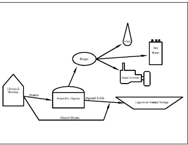
Figure 1. Schematic of AD System
