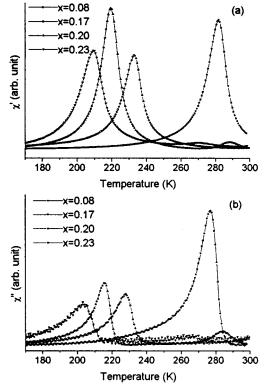
FIG. 4. In-phase (a) and out-of-phase (b) ac susceptibility vs temperature of  $PrCo_{3-x}Si_x$  for  $x=0.08,\ 0.17,\ 0.20,\ and\ 0.23.$
