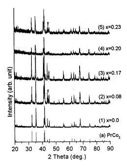
FIG. 1. X-ray diffraction scans for the  $\text{PrCo}_{3-x}\text{Si}_x$  samples: (1) x = 0.08, (2) 0.17, (3) 0.20, and (4) 0.23, and (a) peak intensities for  $\text{PrCo}_3$  from (JCPDS) database.
