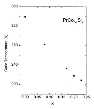
FIG. 5. Estimated Curie temperature of  $PrCo_{3-x}Si_x$  as a function of x.
