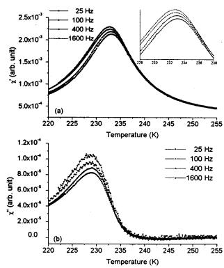
FIG. 3. Frequency dependence of in-phase (a) and out-of-phase (b) ac susceptibility of  $PrCo_{3-x}Si_x$  for  $x\!=\!0.17$  and  $\nu\!=\!25$ , 100, 400, and 1600 Hz. The inset shows the cusps in more detail.
