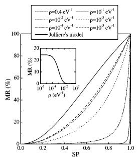
FIG. 3. Magnetoresistance as a function of the spin polarization of the electrodes for various values of  $\rho$  and  $\delta$ =0.04 eV. The solid line shows the result for Julliere's model that is indistinguishable from the result for  $\rho$ =10<sup>-5</sup> eV<sup>-1</sup> and  $\delta$ =0. The inset shows MR versus  $\rho$  for P=0.5 and  $\delta$ =0.04 eV.
