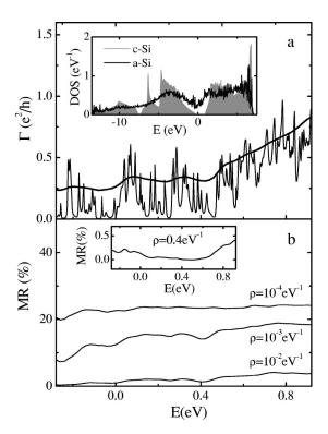
FIG. 2. Conductance (a) and magnetoresistance (b) versus electron energy for P = 0.5.  $\Gamma$  is plotted for  $\delta = 0$  (thin line) and  $\delta = 0.04$  eV (thick line) for  $\rho = 0.4$  eV<sup>-1</sup>. The inset in (a) shows the DOS for c-Si and a-Si. MR is plotted for various values of  $\rho$  and  $\delta = 0.04$  eV. The Fermi energy lies at zero.
