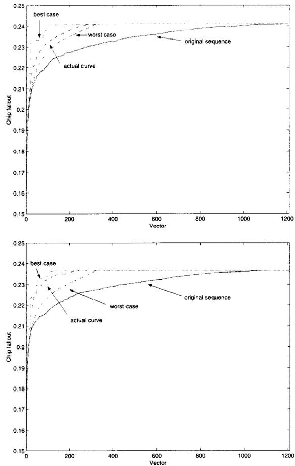
**Figure 5. Simulation results for low clustering (top,  $c = 2.8$ ) and high clustering (bottom,  $c = 20$ ) of faults. Actual cost curves for the sort sequence are well above the original curve in the worst case, and may approach the curve in the best case in high fault clustering case.**
