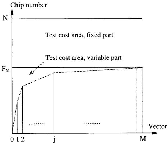
**Figure 1. The test failure curve as the test cost curve. The cost area includes two parts: the fixed part for the good chips, and the variable part for the defective chips. The latter varies for different order of test-vector application.**
