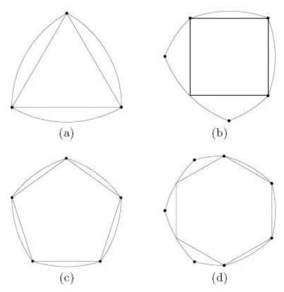
The Reuleaux polygons are named for the 19<sup>th</sup> Century German mechanical engineer Franz Reuleaux. Reuleaux was a brilliant engineer. He created over 300 models of simple machines and is remembered for the Reuleaux triangle. The Reuleaux triangle is a curve with constant width that has been used in Mazda Car Company's rotary engines. The Mazda RX-7 is equipped with a rotary engine. The rotary engine reduces vibration and noise because there is no opportunity for metal surfaces to strike.
