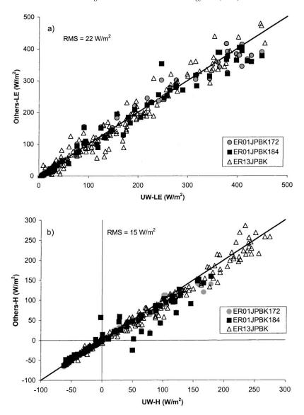
Fig. 3. One-to-one graph of EC system comparison between UW Campbell Scientific (CSI) type and other CSI type systems: (a) latent heat flux (LE) measurements, and (b) sensible heat flux (H) measurements.
