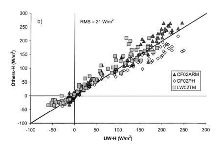
Fig. 4. One-to-one graph of EC system comparison between UW CSI type and non-CSI (mixed) type systems: (a) LE measurements, and (b) H measurements.
