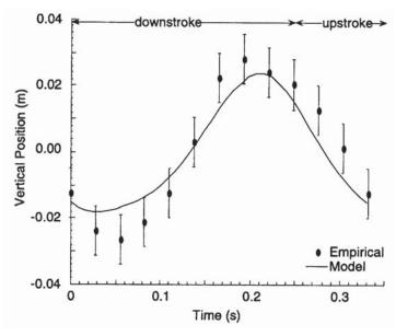
Figure 6.9. Comparison of the vertical oscillations of the bat's center of mass over one wingbeat cycle as computed from the model (*solid line*) and as measured directly from wind-tunnel film footage (*filled circles*; *bars* represent 2 SDs).
