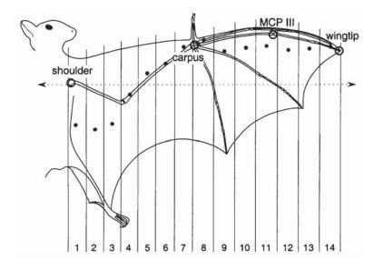
**Figure 6.7.** Plan-view of the ventral surface of the wing of a *Pteropus poliocephalus* held in a position similar to that of mid-downstroke, showing the subdivision of the wing into 14 chordwise strips for the purpose of computer modeling. The filled circles indicate the locations of the centers of masses of these strips relative to a reference line connecting the two shoulders. The open circles indicate anatomical locations used as landmarks for collecting kinematic data.
