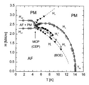
FIG. 1. H-T-phase diagram of FeBr $_2$  (Ref. 4), where H is the applied axial magnetic field. The phase lines  $H_c$ ,  $H_{c1}$ ,  $H_{c2}$ ,  $H_-$ , and  $H_+$  vs T refer to measurements of M vs H (open squares), M vs T (open circles), and  $\chi''$  vs T (solid triangles).  $H_1$  and  $H_1'$  vs T denote the positions of the spikes found by specific heat (open diamonds) (Ref. 10) and off-axis magnetization measurements (solid circles; see Fig. 3), respectively.
