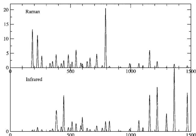
FIG. 20. Vibrational spectrum for the SE1 structure.
