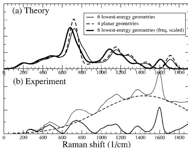
FIG. 22. (a) Computed Raman spectrum for a Boltzmann distribution of the six lowest-energy  $C_2B_{10}$  clusters (solid line), those including only the planar structures (dashed line), and the six lowest-energy clusters with frequency scaled by 0.94 (heavy solid line) and (b) experimental data for a  $C_2B_{10}H_\epsilon$  film (thin solid line), fitted Gaussian background (dashed line), and data with background removed (thick solid line).
