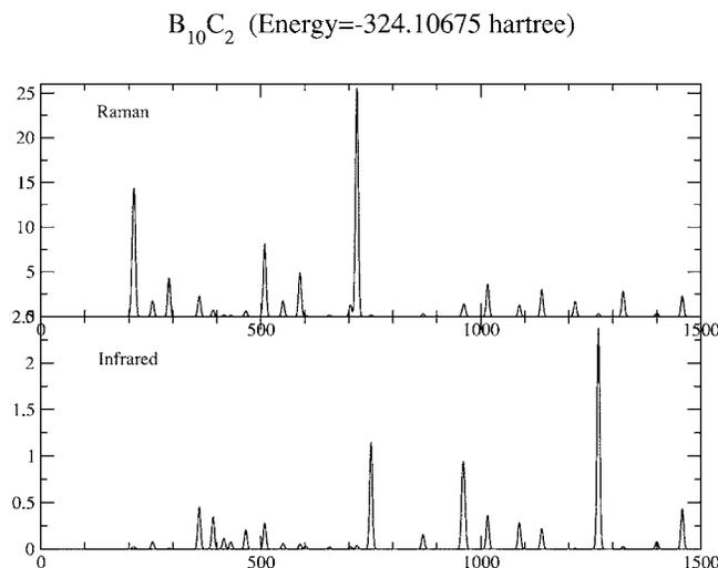
FIG. 10. Vibrational spectrum for the GS structure.
