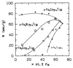
FIG. 2. Spontaneous magnetization measured at 6 K of amorphous  $Fe_x Co_{70-x} Ti_{30}$ ,  $Fe_x Ni_{70-x} Ti_{30}$ , and  $Fe_x Cu_{70-x} Ti_{30}$  as a function of Fe content.
