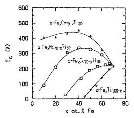
FIG. 4. Magnetic ordering temperature ( $T_c$ ) of amorphous Fe<sub>x</sub>Co<sub>70-x</sub>Ti<sub>30</sub>, Fe<sub>x</sub>Ni<sub>70-x</sub>Ti<sub>30</sub>, Fe<sub>x</sub>Cu<sub>70-x</sub>Ti<sub>30</sub>, and Fe<sub>x</sub>Ti<sub>100-x</sub> as a function of Fe content.
