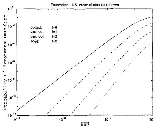
Figure 5: Performance of a (15,5) BCH code used to protect a single low priority request mini-slot
