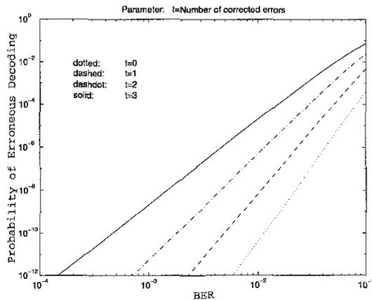
Figure 4: Performance of a (7,1) repetition code used to protect a single high priority request mini-slot or acknowledgement mini-slot
