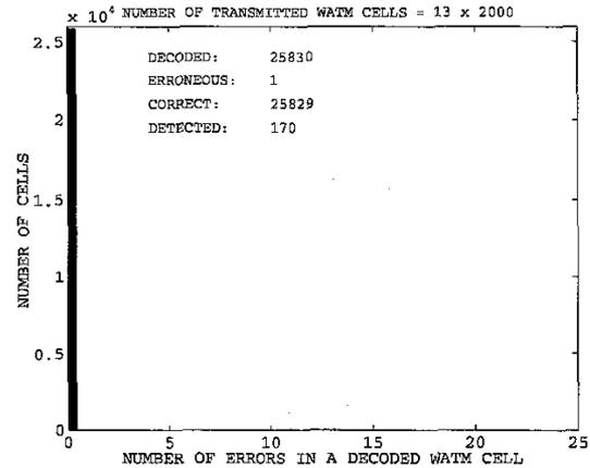
Figure 3: Histogram of the numbers of errors in a WATM cell after decoding for all 13 channels.
