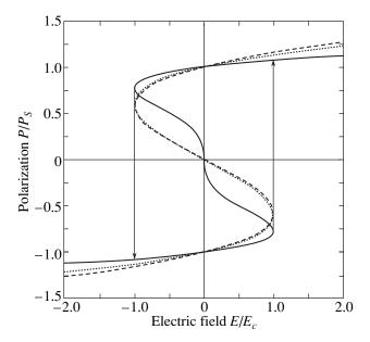
**Fig. 1.** Theoretical ferroelectric hysteresis loops from the first-order Landau–Ginzburg model (solid line), second-order Landau–Ginzburg model (dashed line), and Ising–Devonshire model (dotted line).
