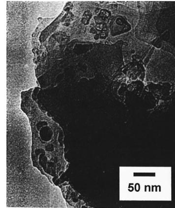
FIG. 3. Transmission electron micrograph of  $\text{SmCo}_5$  milled for 2 h. The powders were encased in epoxy and microtomed prior to imaging.
