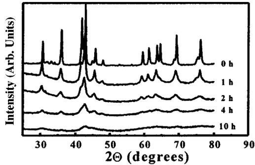
FIG. 1. X-ray-diffraction patterns for mechanically milled  $\text{SmCo}_5$  powders for times of (top to bottom) 0, 1, 2, 3, 4, and 10 h.
