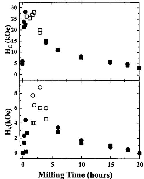
FIG. 6. The dependence of the coercivity ( $H_c$ ) and hysteresis loop shift ( $H_s$ ) on milling time for samples measured at 100 K (squares) and 5 K (circles). Open symbols represent measurements in which the hysteresis loop was not fully saturated.
