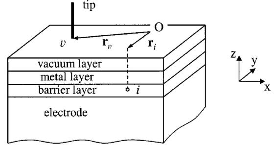
FIG. 2. Geometry in the calculations. The magnetic tunnel junction is infinite in the lateral  $xy$  direction. An impurity is introduced in the barrier layer at site  $i$ . Index  $v$  denotes the site in the vacuum layer which is coupled to the tip.  $\mathbf{r}_v$  and  $\mathbf{r}_i$  are the transverse coordinates of sites  $v$  and  $i$ .
