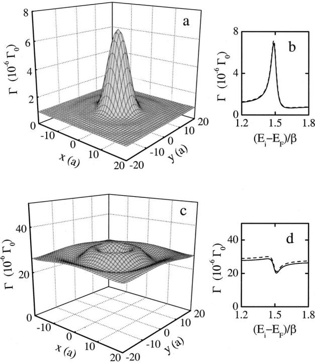
FIG. 3. Lateral distribution of the conductance calculated at  $E_i - E_F = 1.49\beta$  for  $L_m = 10a$  (a) and  $L_m = 20a$  (c) and the respective dependence of the conductance on the impurity energy (b), (d) calculated exactly (solid lines) and using Eq. (7) (dashed lines). Parameters of the model are as follows:  $E_t - E_F = 0$ ,  $E_e - E_F = E_m - E_F = 3\beta$ ,  $E_b - E_F = 6.2\beta$ ,  $L_b = 5a$ , and  $L_v = 10a$ .
