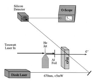
FIG. 3. Experimental setup used for measuring the microsecond decay of the  $e^-_{\rm aq}$  in water. The time resolution (determined by the detector) was 0.3  $\mu$ s. A 100  $\mu$ m thick aluminum foil was used to filter out all of the 1053 nm photons.
