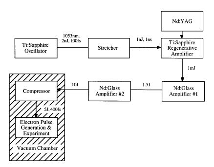
FIG. 1. Block diagram of the laser system. The laser is capable of generating up to 5 J in a 400 fs pulse centered at 1053 nm. The compressor and all subsequent optics are kept under a vacuum of a few mbar. The repetition rate of the laser is 1 shot/10 min.
