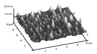
FIG. 1. AFM image of a typical  $Mg_xZn_{1-x}O$  surface.
