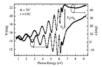
FIG. 3. Experimental (symbols) and best-model calculated ellipsometry data for a  $Mg_xZn_{1-x}O$  film deposited on c-plane sapphire (CP-MDF: solid lines; CA-MDF: dashed lines). Vertical bars denote transition energies of CP contributions in the near-band-gap spectral region  $E_0$  and  $E_0+\Delta_0$ .
