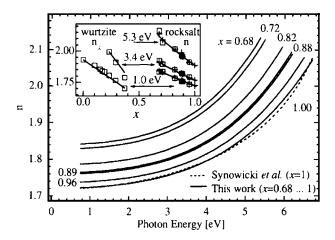
FIG. 5.  $Mg_xZn_{1-x}O$  index of refraction n according to Eq. (7) and parameters in Table II (solid lines). For comparison, data reported by Synowicki and Tiwald (Ref. 30) for x=1 are included (dashed lines). The inset depicts n for individual photon energies calculated from the best-model CP-MDF (open squares), the best-model CA-MDF for each sample individually (crosses), and for all samples simultaneously (solid lines). Data for the wurtzite part were taken from Ref. 2.
