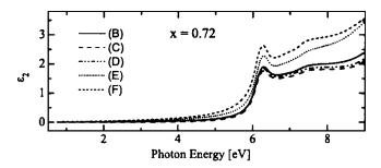
FIG. 2. Spectra of  $Mg_xZn_{1-x}O$  dielectric functions  $\varepsilon_2$  obtained from the MDF analysis using the surface over layer models (B)–(F) listed in Table I exemplarily for x=0.72.
