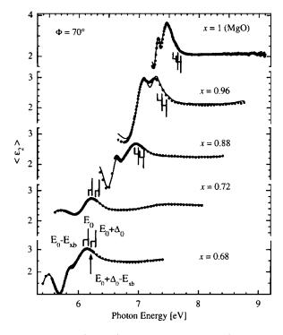
FIG. 4. Experimental (symbols) and best-model calculated (CP-MDF: solid lines)  $\langle \varepsilon_2 \rangle$  spectra for various  $\mathrm{Mg_x} Z \mathrm{n_{1-x}} \mathrm{O}$  films deposited on c-plane sapphire. Brackets with vertical bars indicate the transition energies  $E_0$  and  $E_0+\Delta_0$  (long bar), and their respective exciton resonance  $E_0-E_{\mathrm{xb}}$  and  $E_0+\Delta_0-E_{\mathrm{xb}}$  (short bar).
