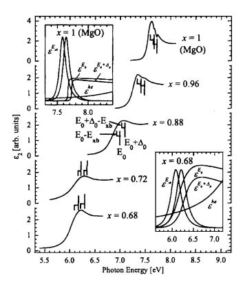
FIG. 6. Calculated  $\varepsilon_2$  spectra applying for the used model with the CP-MDF and surface over layer approach described above for the  $\mathrm{Mg}_x\mathrm{Zn}_{1-x}\mathrm{O}$  samples in Fig. 4. Brackets with vertical bars indicate the transition energies  $E_0$  and  $E_0+\Delta_0$  (long bar), and their respective exciton resonances  $E_0-E_{xb}$  and  $E_0+\Delta_0$  (short bar), and insets display their individual model contributions exemplarily for x=1 and x=0.68.
