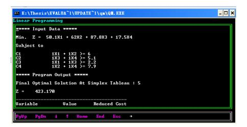
Figure 7 displays the output results of demonstration of linear programming by AB: QM. We can see the minimum cost Z is \$423.17.
