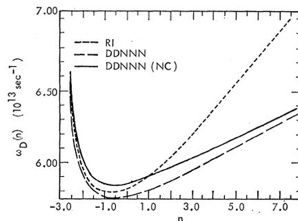
FIG. 4. Plots of the moment function  $\omega_D(n) = \left[ \frac{1}{3}(n+3)\mu_n \right]^{1/n}$ , where  $\mu_n$  is the  $n$ th moment of the frequency spectrum, against  $n$  for the three models, with 0°K input parameters.
