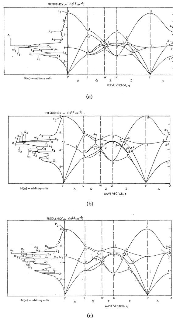
FIG. 2. Results as for Fig. 1 with input parameters appropriate to 300°K. (a) The RI model, sample of 8000  $q$  vectors; (b) the DDNNN model, sample of 64 000  $q$  vectors; and (c) the DDNNN(NC) model, sample of 8000  $q$  vectors.
