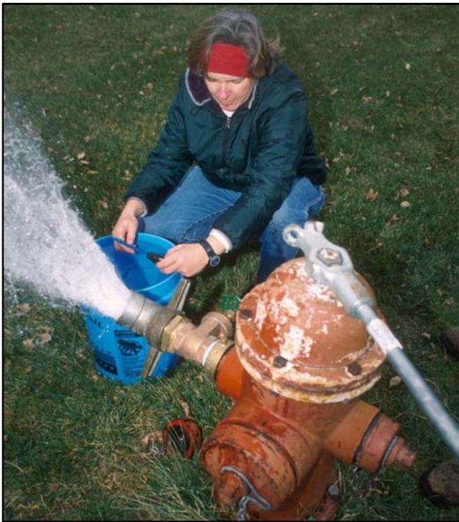
UNL School of Natural Resources project coordinator Lynne Klawer monitors pH and temperature during a water main flush at Stromsburg that is part of a project to help small communities find lower-cost ways to reduce or eliminate arsenic in drinking water (IANR photo: Brett Hampton).
