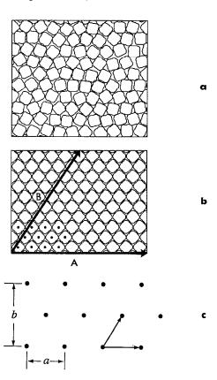
FIG. 4. (a) A snapshot of the high temperature (T=0.200) phase. (b) A snapshot of the low temperature (T=0.001) phase. A and B indicate vectors used to generate the periodic space. (c) A diagram illustrating b and a, which for the systems studied, correspond to next-nearest and nearest neighbor distances, respectively. Average primitive lattice vectors, shown as bold arrows, may be derived directly from the periodic space vectors A and B.
