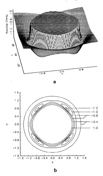
FIG. 3. (a) Reduced potential energy surface plotted as a function of  $r_{ij}$  and  $\phi_i$ ,  $\phi_j = \pi/4$  and  $\phi_{ij} = 0$ . The hard core of the potential is cropped for clarity. (b) A contour plot of the potential energy surface. The contour lines along the hard core resemble the shapes drawn in Figs. 1 and 2.
