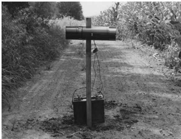
Figure 1. Infrared transmitting unit (left) and receiving unit (right) of the deer-activated bio-acoustic frightening device along the edge of a cornfield.
