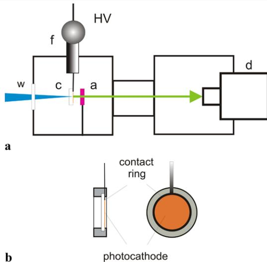
**Fig. 1** **a** Basic layout of the electron gun. *w*: window for trigger laser; *c*: cathode holder; *a*: anode; *f*: high-voltage feedthrough, *d*: detector with sensitized fiber extension. The edge length of the two cubes is 20 cm, the length of the drift tube is 10 cm. The distance from the anode to the detector was 30 cm. **b** Detailed drawing of the cathode assembly in side and front view
