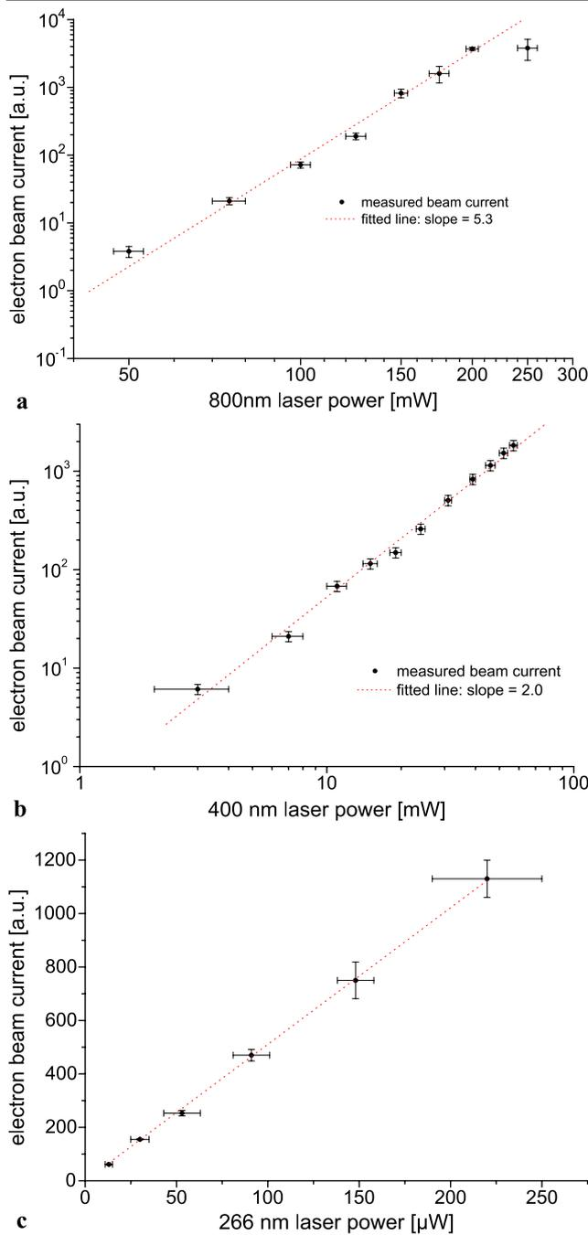
**Fig. 2** **a** Electron beam current vs. fundamental laser power. The data are fitted with a power law with slope 5.3 indicating above threshold emission. **b** Electron beam current vs. laser power for 400-nm laser light (second harmonic). A power law with a power of two describes the dependence. **c** Electron beam current vs. third harmonic laser power. A linear correlation is obtained
