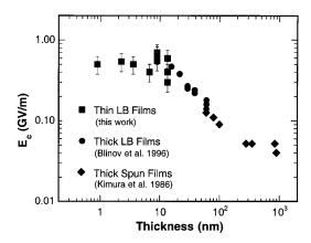
FIG. 3. The finite-size effect for the coercive field  $E_C$  in P(VDF-TrFE) over three decades in thickness, from 1 nm to 1  $\mu$ m. The diamonds are data from P(VDF-TrFE 65:35) films made by solvent spinning [11]. The circles and squares are data from P(VDF-TrFE 70:30) films made by LB deposition reported previously [23] (circles) and for the first time in this study (squares).
