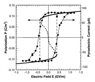
FIG. 1. The theoretical polarization P(E) at 25 °C (thick-solid line) of P(VDF-TrFE 70:30) calculated from the LG expression [Eq. (3)] and the hysteresis in the pyroelectric response at 25 °C (circles) in a 30-ML LB film of P(VDF-TrFE 70:30). The solid lines in the P(E) response represent stable or metastable minima in the free energy density [Eq. (1)], but the dotted line joining them represents an unstable maximum.
