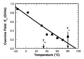
FIG. 2. The intrinsic coercive field of a 20-ML LB film of P(VDF-TrFE 70:30). The solid line is the LG expression [Eq. (3)] calculated with only one adjustable parameter, the value of the coercive field  $E_{C0}$  at the temperature  $T_0 = 33.7\,^{\circ}\text{C}$ .
