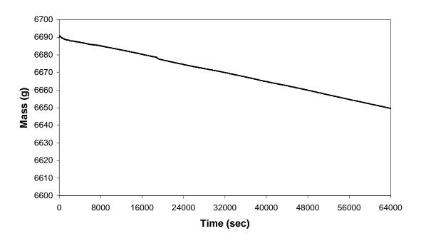
Figure 5. Sample weight loss history of fully wetted plaster-covered aluminum ham testing (replication 2) during air drying (initial core temperature 6.24°C, air velocity 1.11 m/s, relative humidity 82.06%, initial mass 6,690.9 g).
