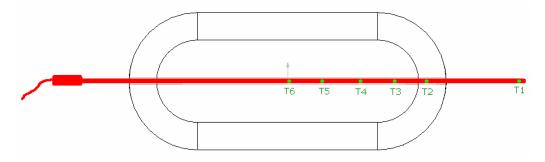
Figure 2. Placement of Custom-built multisensor temperature profiling probe (Omega Engineering, Inc.); thermocouples T1-T6 inside of aluminum ham model.
