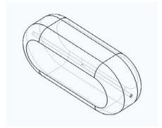
Figure 1. Drawing of Aluminum Ham Model (created in SolidWorks $^{\otimes}$  2001). Dimensions: 23.5 cm long  $\times$  8.9 cm thick  $\times$  12.7 cm wide.
