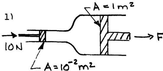
For the hydraulic system shown, find the force on the large piston.
