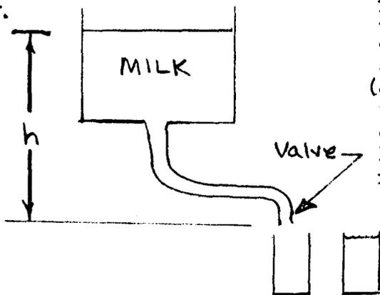
Milk containers on an assembly line are being filled from a hose connected to a large reservoir which can be raised or lowered. The automatic valve (area =  $10^{-4} \text{ m}^2$ ) on the hose opens for  $3 \text{ s}$  to fill the milk containers with  $10^{-3} \text{ m}^3$  of milk ( $\rho_{\text{milk}} = 10^3 \text{ kg/m}^3$ ). Find the height required so that proper amount of milk is dispensed into each container.
