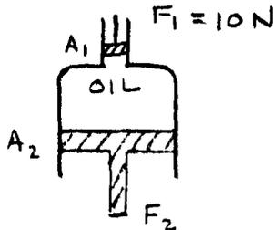
You are designing a hydraulic punch press that requires a force  $F_2$  on the punch of  $10^6 \text{ N}$ . If the oil pump can deliver a force of  $10 \text{ N}$ , what will you choose for the ratio of the areas of the large and small pistons?
