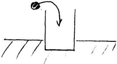
A beer can floats in the water. The can is  $.02 \text{ m}$  in radius and  $0.1 \text{ m}$  long. The empty can has a mass of  $0.03 \text{ kg}$ . How many  $0.01 \text{ kg}$  mass stones must be dropped into the can to sink it?
