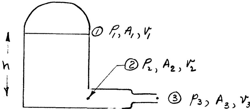
Water in a closed tank flows out a valve at  $A_3$  when the valve is turned on. What absolute pressure  $P_1$  is needed to produce a flow velocity  $V_2 = 10 \text{ m/s}$  with the valve open?
