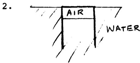
An inverted beer can weighing  $10^{-2}$  N is found barely to float as shown. Find the volume of air trapped in the can. (You may neglect the mass of the air.)
