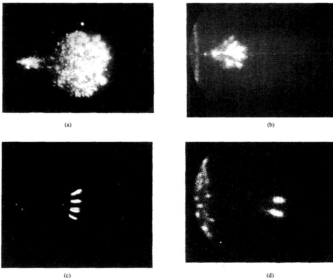
Fig. 1. Figure showing streamers in pure  $N_2$ , (a) and (b), and mixtures containing 15%, (c) and 1%, (d),  $O_2$ . Streamers in (a) and (c) are propagating toward the cathode, those in (b) and (d) toward the anode. In all cases, the initiating point is at the left of the photo. The total horizontal distance shown varies a little between photos and is about 16 cm. The features at the far left in (b) and (d) are due to streamers initiated at the edge of the charged electrode.
