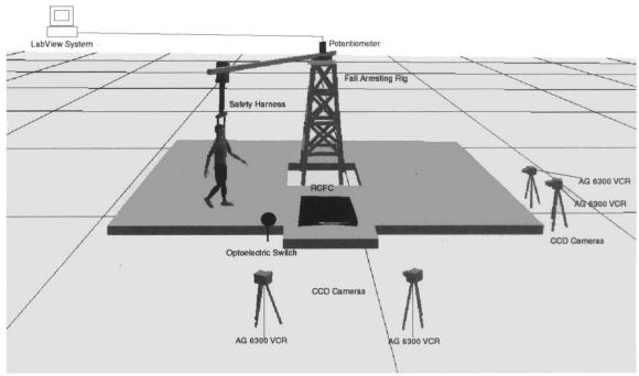
**Figure 2.** Field layout of the experiment, including fall-arresting rig, potentiometer interfaced with the LabView system, safety harness, force platforms, optoelectric switch, CCD cameras (4), AG 6300 VCR (4), and remote control floor changer (RCFC) units with baseline carpet floor material
