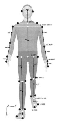
**Figure 3.** Locations of marker placements and internal landmarks used to generate whole-body center of mass and calculations of slip parameters.
