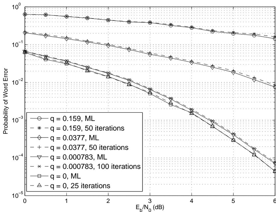
Figure 5.9: A comparison of word-error rates for the  $[32, 16, 8]$  Reed-Muller code on the binary asymmetric channel for several values of  $q := P(0 | 1)$ . A value of 0 for  $q$  indicates the Z-channel. The horizontal axis measures  $p := P(1 | 0)$ .
