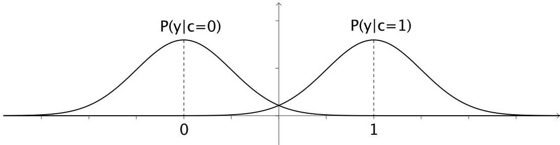
Figure 2.6: The additive white Gaussian noise channel.
