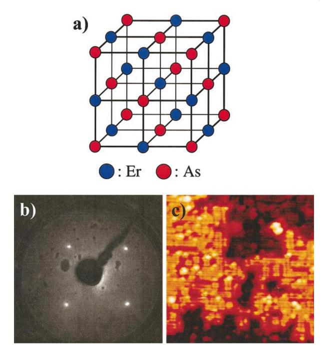
FIG. 1. (Color) The structure (a) of ErAs(100) is shown together with the LEED (b) of the stoichiometric ErAs(100) surface grown on GaAs(100) for an electron kinetic energy of 58.5 eV. The *in situ* image of STM of the growth of ErAs(100) film  $(25 \times 25 \text{ nm})^2$  is also shown (c), and was acquired with a -2.5 V bias.
