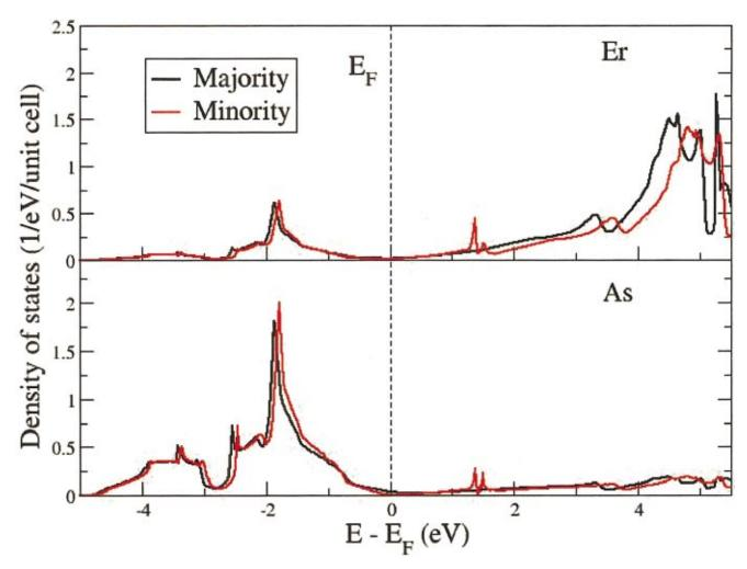
FIG. 3. (Color) The Er 5d density of states (a) and As density of states (b) near the Fermi energy from LSDA+U calculations of ErAs(100) (see the text). U = 8.6 eV was used.
