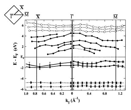
FIG. 6. The experimental band structure of the ErAs(100), along  $\overline{\Gamma X}$  and  $\overline{\Gamma M}$  high-symmetry lines of the surface Brillouin zone compiled from combined photoemission (bottom) and inverse photoemission (top) results. The high-symmetry points and directions of the surface Brillouin zone of the crystal is indicated in the inset at the top of the figure. Bands with a strong 4f weight are indicated by the dashed lines.
