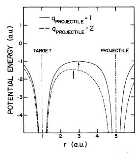
FIG. 1. Potential energy plots for  $\phi = -(q_T/|1-r|)$   $-(q_p/|5-r|)$ , where  $q_T$  and  $q_p$  are the final target and projectile charges, respectively. The target is placed at r=1 for convenience.
