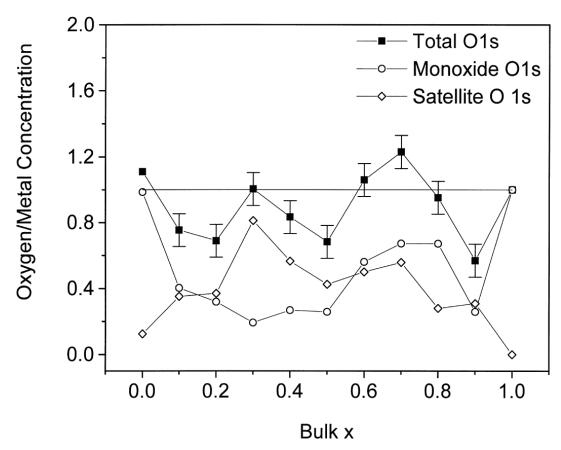
**Figure 12.** XPS determination of oxygen to total metal concentration ratios as a function of the bulk x for the  $Mn_xCo_{1-x}O$  solid solutions after sputtering. Data include total oxygen concentration (•), lattice oxygen 529.4 eV component ( $\circ$ ) and "defect" 531.3 eV component ( $\diamond$ ). For clarity, error bars are placed only on total oxygen data; other data in the plot have comparable precision.
