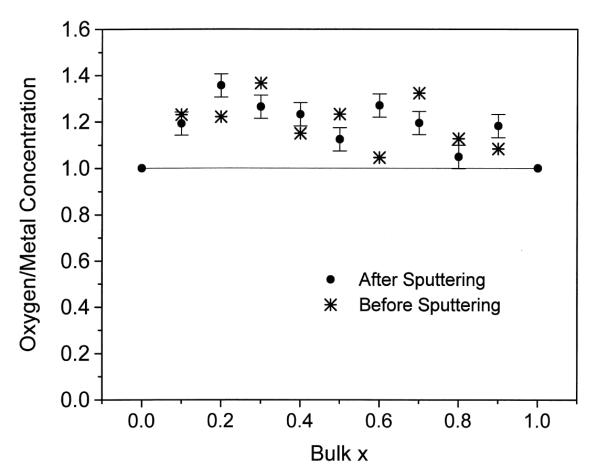
**Figure 3.** Auger determination of oxygen to total metal concentration ratio as a function of the bulk x value for the solid solutions before (\*) and after (•) sputtering. For clarity, error bars are placed only on data after sputtering; data before sputtering have comparable precision.
