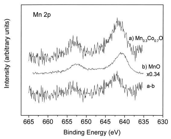
**Figure 8.** Illustration of the Mn 2p XPS subtraction procedure for removing the Mn $^{2+}$ component to the Mn $_{0.3}$ Co $_{0.7}$ O spectrum.
