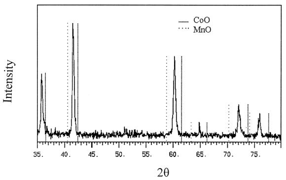
**Figure 1.** Powder X-ray diffraction (XRD) of the  $Mn_{0.5}Co_{0.5}O$  solid solution sample, taken with Cu K $\alpha$  radiation. Light dashed lines represent positions for pure MnO and heavy dashed lines represent positions for pure CoO.
