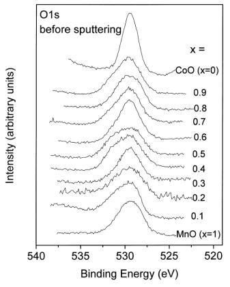
**Figure 9.** XP O 1s spectra as a function of bulk *x* for the "asintroduced" solid solutions.
