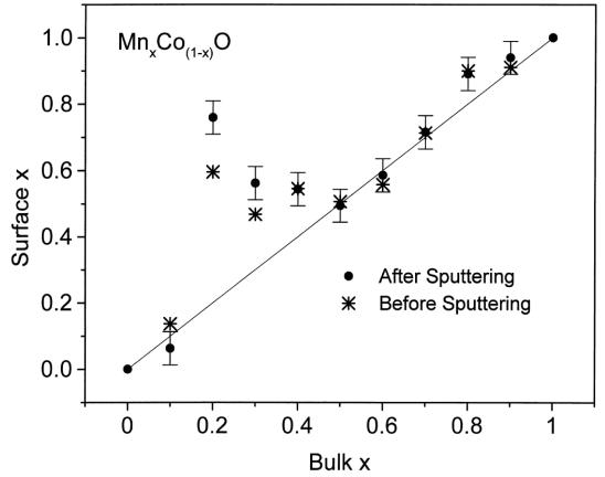
**Figure 4.** XPS determination of surface x composition as a function of the bulk x value for solid solutions before (\*) and after (•) sputtering. For clarity, error bars are placed only on data after sputtering; data before sputtering have comparable precision.
