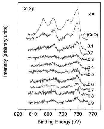
**Figure 5.** Cobalt 2p XP spectrum as a function of the bulk x value. Note that since the solid solution formula is given as  $\mathrm{Mn_xCo_{1-x}O}$ , a smaller x value represents a larger cobalt fraction and pure CoO is represented by x=0. The solid vertical line marks the peak position for the  $2p_{3/2}$  transition at 780.5 eV.
