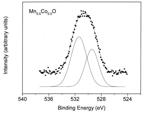
Figure 11. Illustration of the O 1s XPS fitting procedure, discussed in greater detail in the text.
