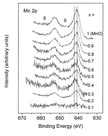
**Figure 7.** Mn 2p XP spectrum as a function of the bulk x value. Note that pure MnO is found for x = 1. The solid vertical lines mark the  $2p_{3/2}$  peak position for each of the two species discussed in the text and are at 640.8 and 642.1 eV.
