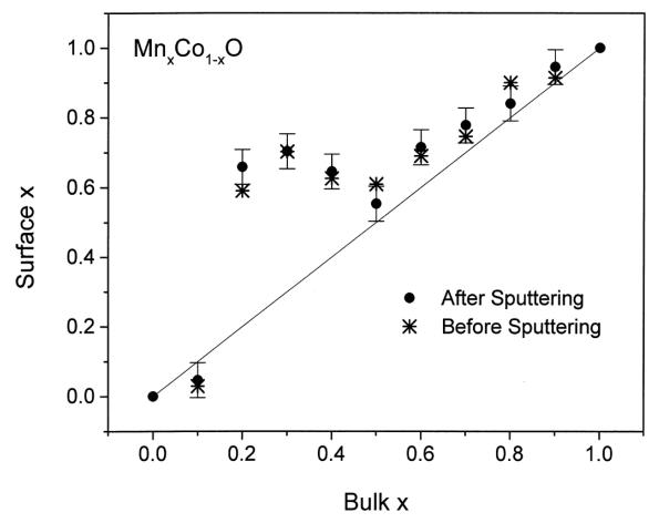
**Figure 2.** Auger determination of surface *x* composition as a function of the bulk *x* value for solid solutions before (\*) and after (•) sputtering. For clarity, error bars are placed only on data after sputtering; data before sputtering have comparable precision.
