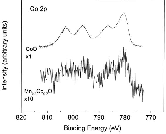
**Figure 6.** Co 2p XP spectrum for  $Mn_{0.3}Co_{0.7}O$  compared to that of pure CoO, showing that the two have similar binding energies and intensive satellite structure expected from the rocksalt monoxide band structure. The  $Mn_{0.3}Co_{0.7}O$  spectral intensity has been increased by  $10^{\times}$  relative to that of the CoO.
