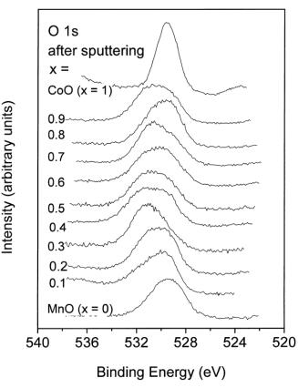
**Figure 10.** XP O 1s spectra as a function of bulk x for the solid solution samples after sputtering.
