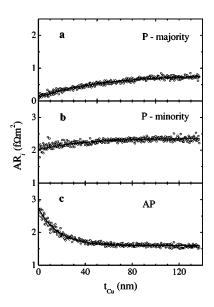
FIG. 3. Spin-resolved resistance of two Co/Cu/Co interfaces separated by disordered Cu layer of thickness  $t_{\text{Cu}}$  for (a) majority-and (b) minority- spin electrons for (c) P magnetization and AP magnetization. Solid lines display fit to the calculated data using Eq. (5).
