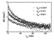
FIG. 5. Calculated  $SR = \sqrt{(AR_{AP})(AR_{AP} - AR_P)}$  vs Cu layer thickness for different values of disorder parameter  $\delta_{int}$  at Co/Cu interfaces.
