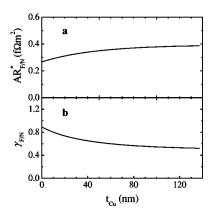
FIG. 4. Parameters of the spin-dependent Co/Cu interface resistance as a function of disordered Cu layer thickness: (a) enhanced interface resistance  $AR_{F/N}^*$  and (b) spin-asymmetry scattering parameter  $\gamma_{F/N}$ .
