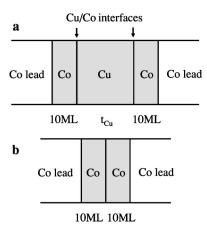
FIG. 1. Geometry used in calculations of the resistances of the Co/Cu/Co trilayer and Co/Cu interfaces. Gray contrast indicates disorder.
