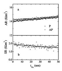
FIG. 6. Resistance for parallel (P) and antiparallel (AP) configuration of (a) a Co/Cu/Co spin valve and SR vs (b) Co layer thickness for  $\delta$ =0.35 eV and  $\delta_{int}$ =1.05 eV assuming that an additional resistor in series is included to fit the resistance measured in Ref. 12. The solid line has the slope of -0.007 f $\Omega$  m<sup>2</sup>/nm, which is the best fit to the experimental data (Ref. 12).
