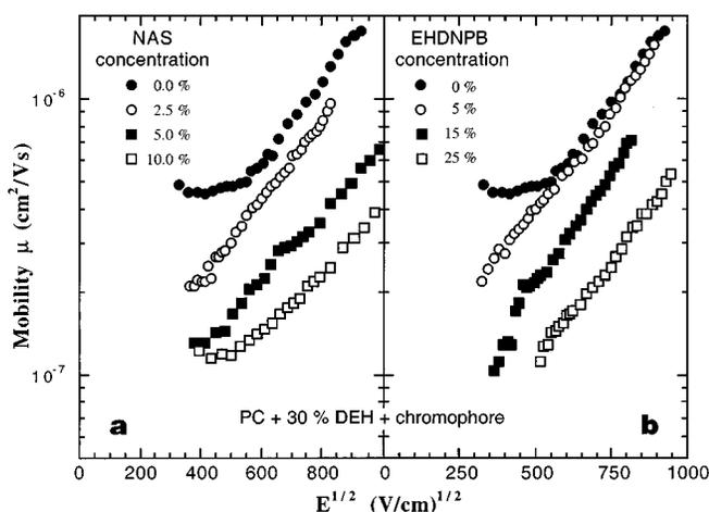
FIG. 7. Logarithm of the mobility vs  $\sqrt{E}$  at 303 K. Compositions PC:30%DEH:X%chromophore for (a) NAS and (b) EHDNPB chromophores.
