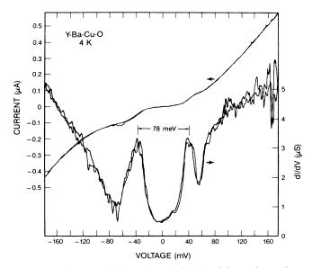
FIG. 2. Current-voltage characteristic and dynamic conductance (dI/dV) showing superconducting gap structure typical of the largest measured in the Y<sub>1</sub>Ba<sub>2</sub>Cu<sub>3</sub>O<sub>9- $\delta$ </sub> break-junction sample.
