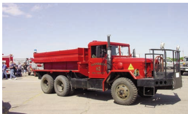
This 2 1/2 ton 6x6 tanker was supplied by NFS to a fire department through the Federal Excess Property Program. The Fire Shop made repairs and brought the tanker up to safety standards and the cooperating fire department (Dannebrog) did the finish work on the vehicle.
