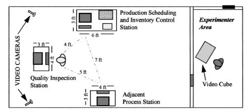
**Figure 1.** Laboratory layout for the experiment including the experimenter area and simulated AMS cell.
