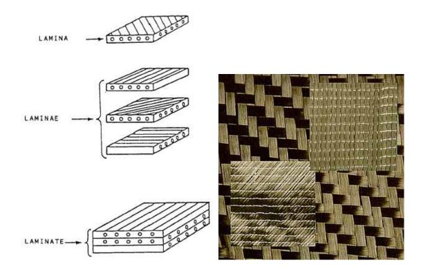
Figure 2.1 Laminated composite materials: (a) Unidirectional reinforcement, and (b) woven fabric reinforcement [2.3-2.4].
