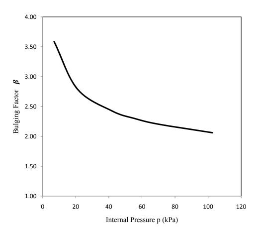
Figure 4.5 Bulging factors for two layers shell [0/30].
