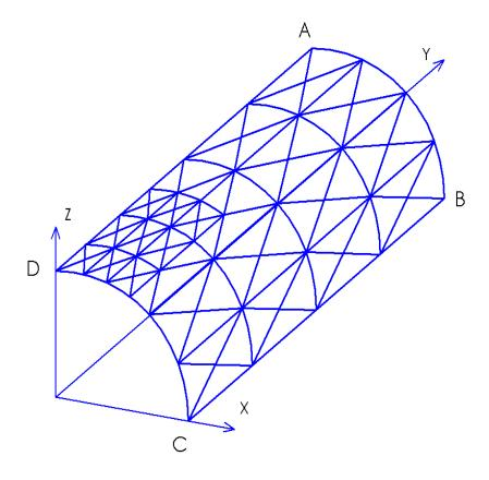
Figure 3.2 Laminated cylindrical shell structure with finite element representation [3.1].
