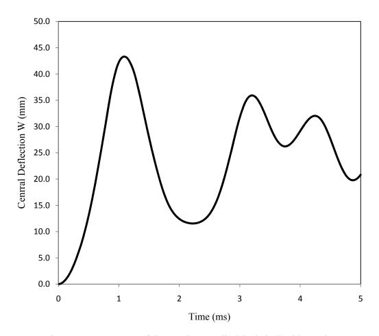
Figure 3.9 Response of the one layer cylindrical shell with crack.
