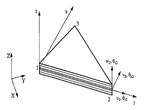
Figure 2.2 Flat triangular laminated composite shell element [2.6].
