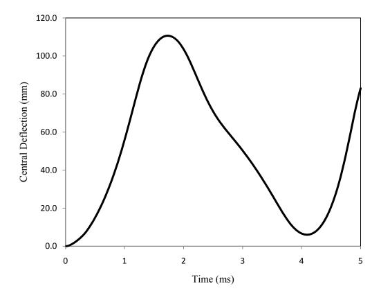
Figure 3.13 Response of four layer cylindrical shell with crack ply arrangement [45/60].
