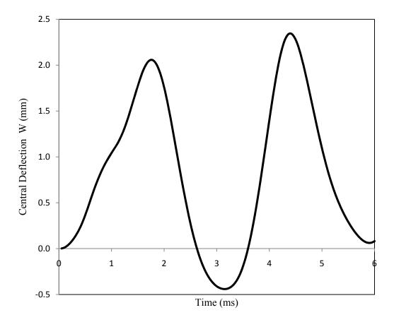
Figure 3.5 Response of the eight layer cylindrical shell
