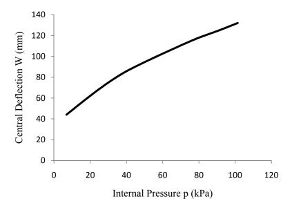
Figure 4.3 Central deflections for two layers shell [0/30].
