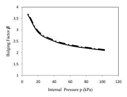
Figure 4.10 Bulging factors for four layers shell with different ply angles:
