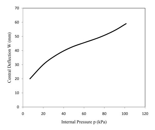
Figure 4.1 Central deflection for single layer shell.
