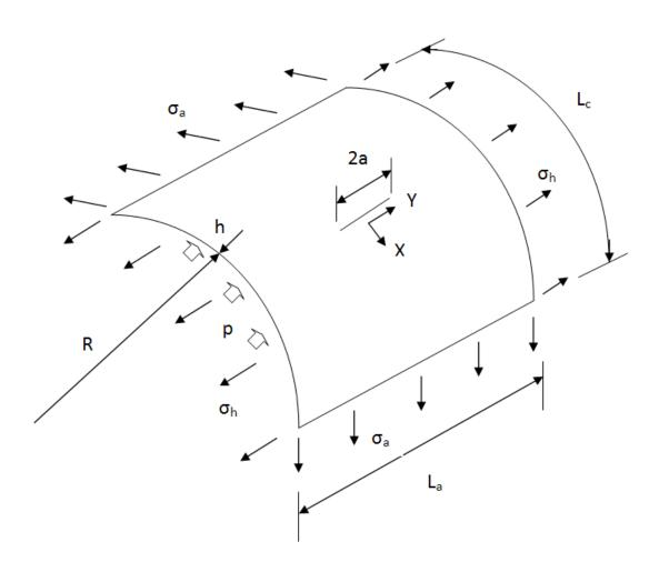
Figure 3.1 Cylindrical shell [3.1].
