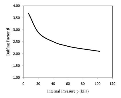
Figure 4.9 Bulging factors for four layers shell  $[0/90]_{sym.}$
