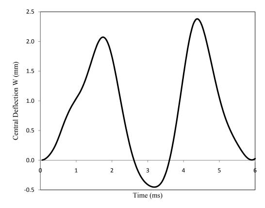
Figure 3.4 Response of the four layer cylindrical shell.
