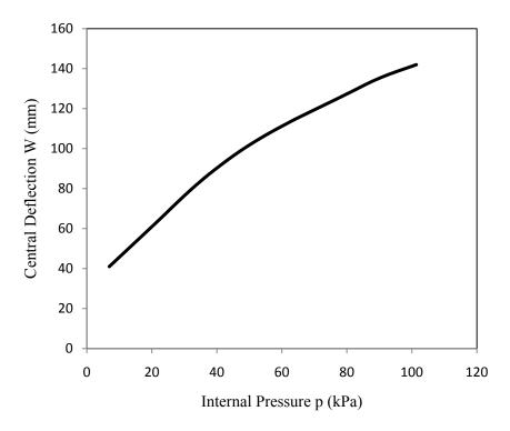
Figure 4.7 Central deflections for four layers shell [0/45] sym.
