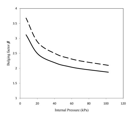
Figure 4.14 Bulging factors for four layers with free-free boundary conditions:
