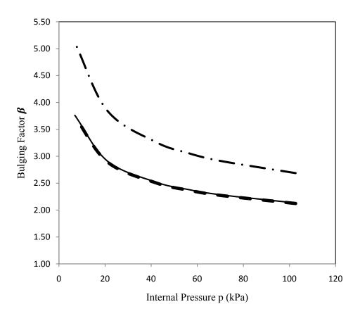
Figure 4.11 Comparison of bulging factors for different number of layers:
