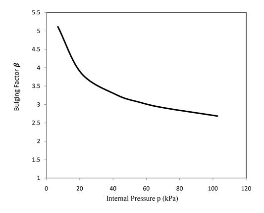
Figure 4.2 Bulging factor of single layer cylindrical shell.
