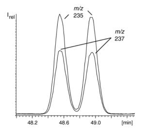
Fig. 2. GC/EI-MS chromatogram (m/z 235 and m/z 237; Chirasil-Dex) of the enantioselective determination of o.p'-DDT in *Eufriesea purpurata*.
