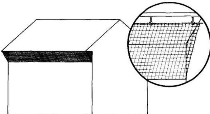
Fig. 1. Netting mounted on building from outside edge of eave down to the side of the building. Insert shows a method of attachment using hooks and dowels.
