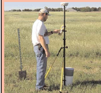
Facilities Operations performs surveying using an RTK (Real Time Kinematics) GPS (Global Positioning System). This system allows Facilities Operations locate infrastructure at the ARDC to within less than one half inch. This system is used to collect GIS (Geographical Information Systems) data for use by other departments.
