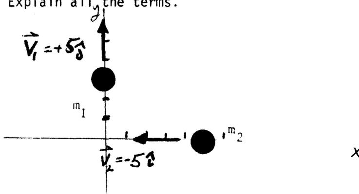
Two particles are moving apart as shown in the figure above. The mass  $m_1$  is 5.0 kg and  $m_2$  is 3.00 kg; at the instant shown they are located at  $3\hat{j}$  m and  $5\hat{i}$  m respectively.
