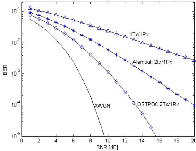
Fig. 2. Bit-error-rate (BER) performance of the developed scheme (OSTPBC) using the code  $Q_1$  combined with QPSK modulation in a slow flat Rayleigh fading channel experiencing random cross-polar scatter compared with the Alamouti scheme and a single transmit/single receive antenna system.
