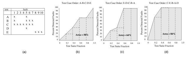
Fig. 4. Example illustrating the APFD measure. (a) Test suite and faults exposed. (b) APFD for Prioritized Suite T1. (c) APFD for Prioritized Suite T2. (d) APFD for Prioritized Suite T3.
