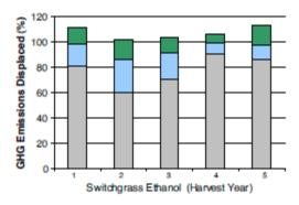
**Figure 3.** Estimated displacement of greenhouse gas (GHG) emissions by replacing gasoline with switchgrass ethanol. Minimum (grey), mean (blue), and maximum (green) percent GHG displacement for each switchgrass harvest year is based on production data from 10 fields. Estimated GHG values include the amount of CO<sub>2</sub> sequestered in the soil (Schmer et al. 2008).
